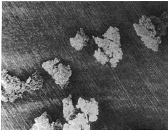
Figure 2 SEM photograph of latex waste filler particles (size 1; magnification ×60).
